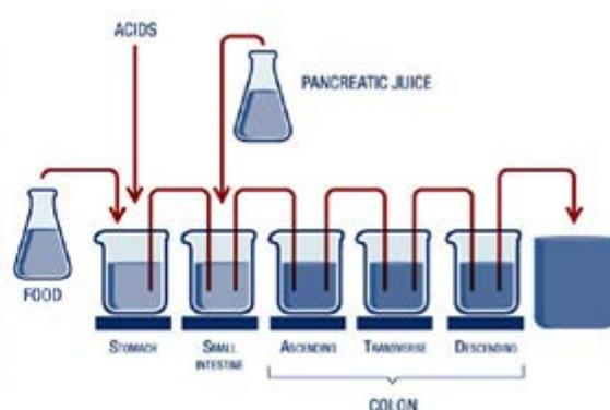
Overview of the TWINSHIME setup, consisting of two parallel SHIME systems. Each SHIME reactor simulates the stomach, small intestine, ascending colon, transverse colon and descending colon.
